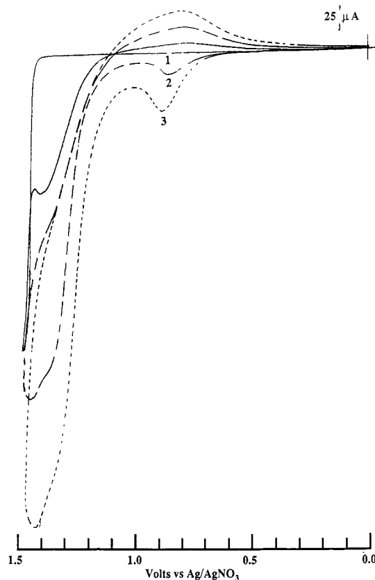
Figure 1. Continuous cyclic voltammograms recorded during the room-temperature polymerization of I on a 0.1-mm 2 Pt disk electrode in acetonitrile containing 0.4 M TBAPF 6 at 20 mV/s. Consecutive scans are shown by the increasing scan numbers.
